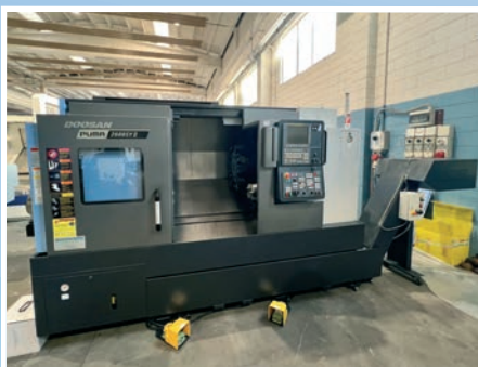
6-Axis lathe with counterspindle, driven tools and Y Axis DOOSAN PUMA 2600SY-II CNC DOOSAN FANUC i- Series
