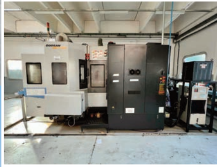
Horizontal machining center with pallet changer DOOSAN ACE HM500 CNC FANUC 181-MB
