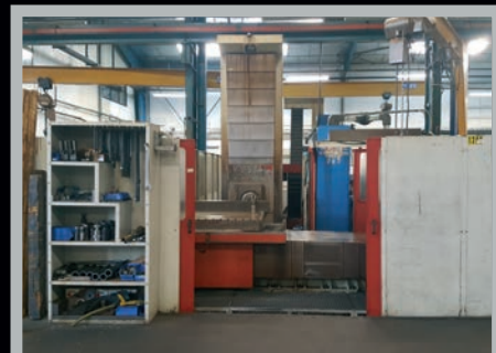
Alesatrice (Boring Machine) SAN ROCCO FMC 110 S , 2100x1600x1600 mm, 3.000 rpm, Tavola 1300x1100 mm, montante a T, CNC HEIDENHAIN TNC 426
