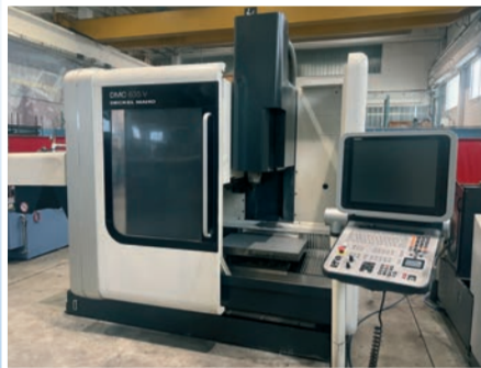
Vertical machining center DECKEL MAHO DMC 635V CNC HEIDENHAIN ITNC-530
