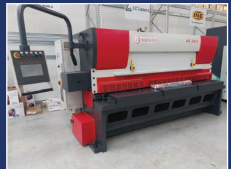
> CESOIA IDRAULICA DENER AS 3000 X 10 MM
