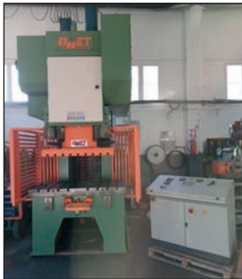
PRESSA OMET 200 TON. PEF-RF 200, DIM. PIANO PRESSA 880 X 1600, DIM. PIANO MAZZA 700 X 1000, LUCE 700
