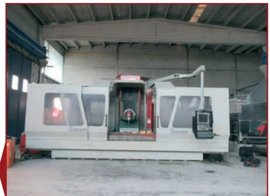
Fresatrice SACHMAN T15 HS X=2005 a banco fisso, 2500x1200x1200, kW 28, 5000 rpm, 2,5°+3°
