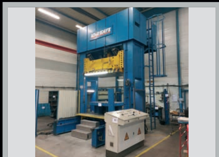
Pressa prova stampi (Die Testing Press) LOIRE SAFE ESSM 200/25 , piani 2500x1500 mm, forza max 2000 Kn, anno 2001
