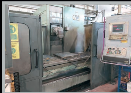
Fresalesatrice (Milling and Boring Machine) FPT SPAZIO 2000 , 2000 x 800 x 1250 mm, testa automatica 2,5°, 4000 rpm, CNC Selca 3045PD
