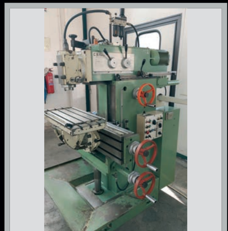
Fresatrice per attrezzeria (Tool Room Milling Machine) C.B.FERRARI M3 , 400x400x450, ISO 40, tavola basculante
