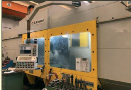
Fresatrice a 5 assi CB FERRARI S630-E580H
