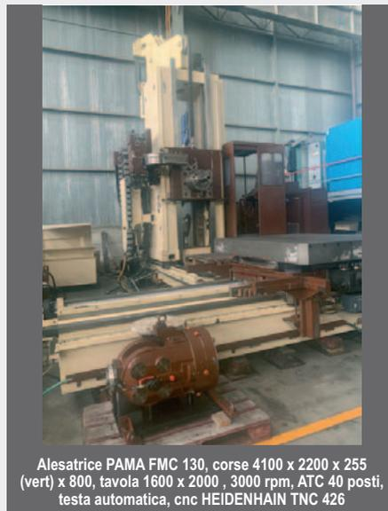
Alesatrice PAMA FMC 130, corse 4100 x 2200 x 255 (vert) x 800, tavola 1600 x 2000 , 3000 rpm, ATC 40 posti, testa automatica, cnc HEIDENHAIN TNC 426
