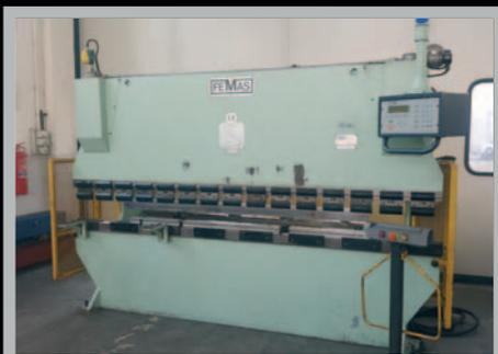
**Pressa piegatrice (Press Brake) FEMAS PI45**, 3050 x 45 ton, CN 3 assi
