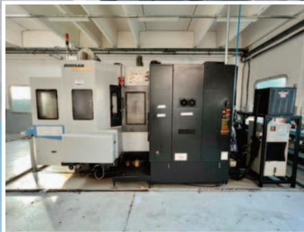
Horizontal machining center with pallet changer
