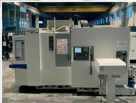
Horizontal machining center with pallet changer
