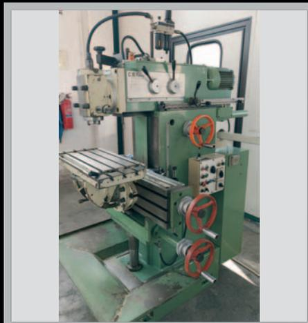
**Fresatrice per attrezzeria (Tool Room Milling Machine) C.B.FERRARI M3**, 400x400x450, ISO 40, tavola basculante
