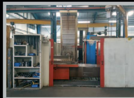
**Alesatrice (Boring Machine) SAN ROCCO FMC 110 S**, 2100x1600x1600 mm, 3.000 rpm, Tavola 1300x1100 mm, montante a T, CNC HEIDENHAIN TNC 426
