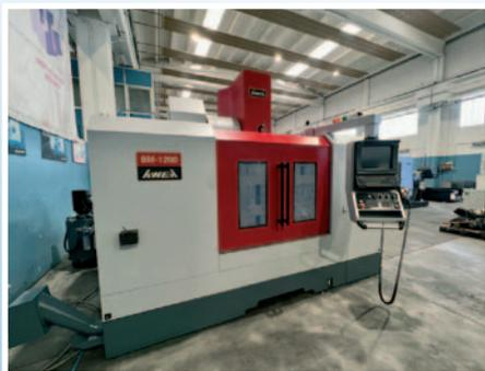
Vertical machining center with 4-Axis TGV 250
