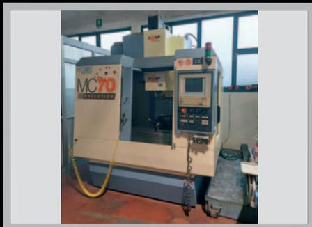
**Centro di lavoro (Machining Centre) FAMUP MC 70 Evolution**, 700x500x640, 24 utensili, 10.000 rpm, CNC SELCA 3045
