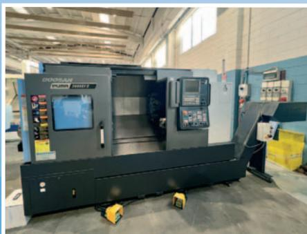
6-Axis lathe with counterspindle, driven tools
