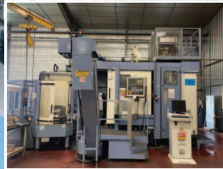
Horizontal machining center with multipallet
