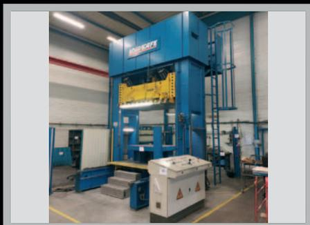
**Pressa prova stamperie (Die Testing Press) LOIRE SAFE ESSM 200/25**, piani 2500x1500 mm, forza max 2000 Kn, 2001
