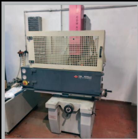
**Elettroerosione (EDM machine) CDM ASTRO 3.40** - 400x300x200+200 mm, vasca 1100x600x460, controllo asse Z
